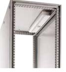
**Description:** Fluorescent lamp equipped with switch electronic starter integrated socket and a protection cap. A male GST 18/3 connector is provided for connection to the power on one side and by a pass-through circuit to a female connector allows a further connection on the other side. An additional connector ST 17/2 allows the activation of the lamp by a door switch.
