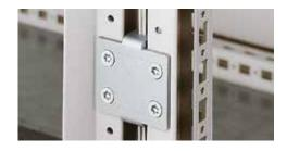
**Description:** Brackets mounted on the outside hole pattern of the frame ensuring a strong and 3 dimensional alignment of the bayed enclosures with "auto spacer" function. This method of baying enclosures also has the advantage of realizing a direct earthing connection between the enclosure frames.
