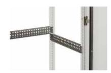
Description: Universal profile for both depth and width fitting on the 25mm DIN hole pattern of the enclosure's frame or in combination with the VB profiles. The 75mm wide profile is equipped with three rows of holes of which one is turned 90°. This makes it possible to mount the CLPF profiles in both directions. The CLPK can be secured by the use of self tapping screws.
